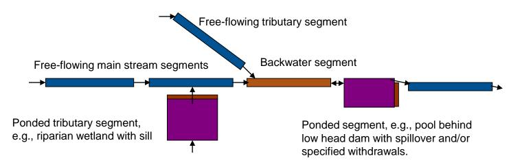
WASP internally calculates flows, volumes, depths, widths in: free-flowing reaches (kinematic wave eq.), ponded reaches (weir overflow eq.), and backwater reaches (dynamic flow eq's.)
